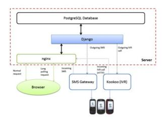
Figure 1: NextDrop System Architecture
